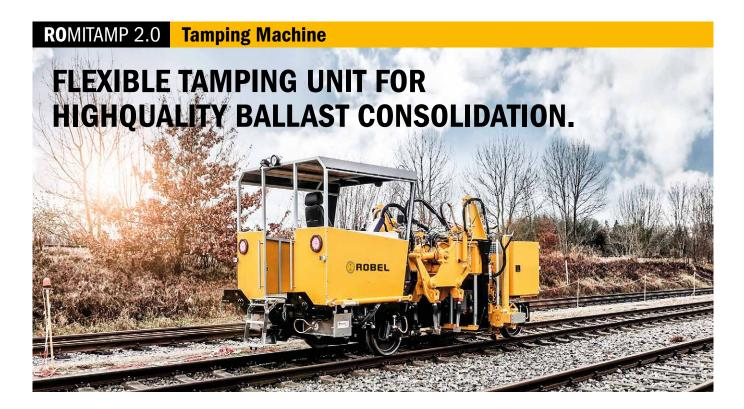
Compact small tamping machine for precise tamping of track sections that are too big for manual correction and too small for economical use of large machines.
