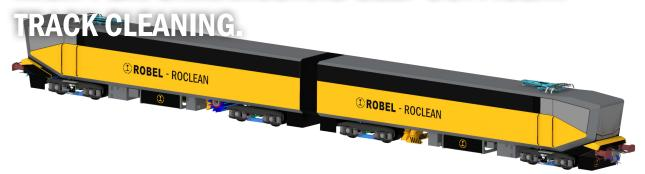
Container based track cleaning system for build on flat wagon with self-sufficient energy supply.
