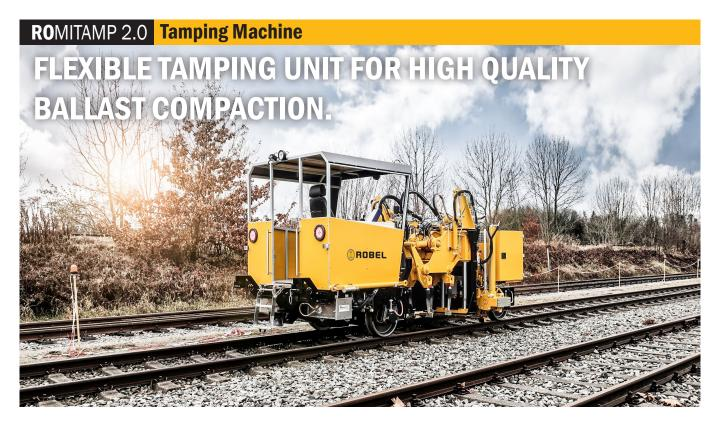
Compact and small tamping machine for precise tamping of track sections, which are to big for manual corrections and to small for economic commitment of large machinery. Application also in terrain, which is difficult to access.
