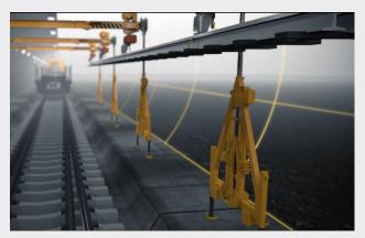
$4. \ \mbox{Hoists}$  then lifting old rails or switches and load on to ROTRAILER. Return to depot.
