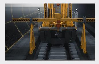
$2. \ Transport \ vehicle \ delivers \ rails \ or \ switches \ to \ worksite.$
