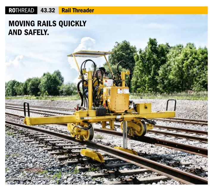
For continuous gradual repositioning of rails to the desired track gauge.
