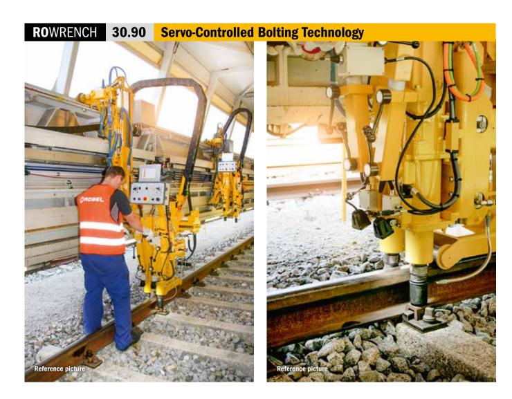
For synchronous tightening and loosening for all wrenching tasks required in track maintenance within ROBEL's ROMIS Mobile Maintenance Unit.
