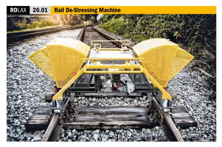
To remove stresses from the rail and establish the nominal length of the rail by striking the rail head on both sides.
