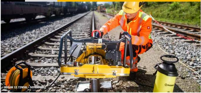
For cutting rails without sparking in new construction and maintenance.
