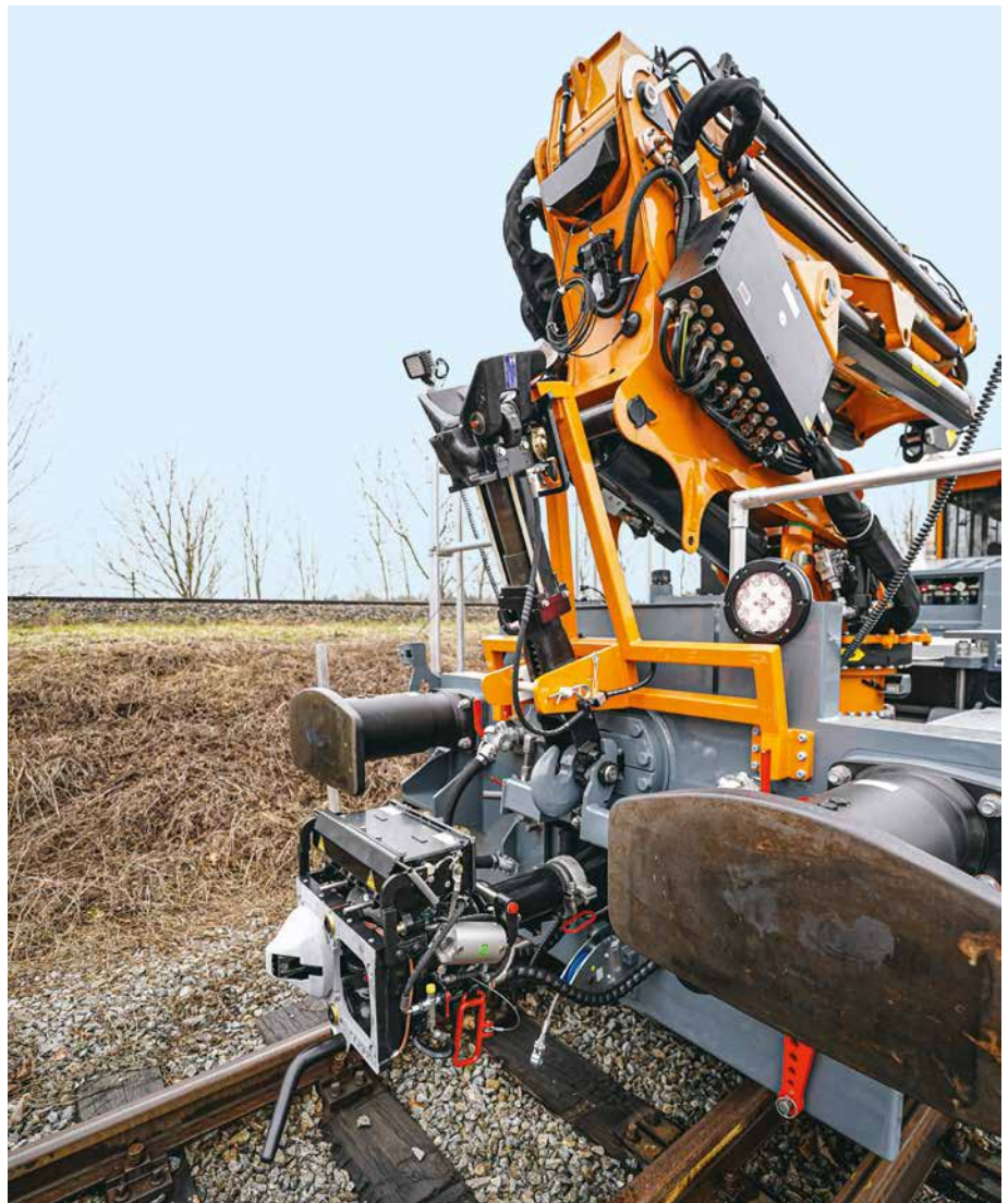
Fig. 6: The vehicles are equipped with a standard draw gear with side buffers, an additional shunting coupler, and a pneumatically lowerable Scharfenberg coupler for operating on underground and heavy rail systems.
