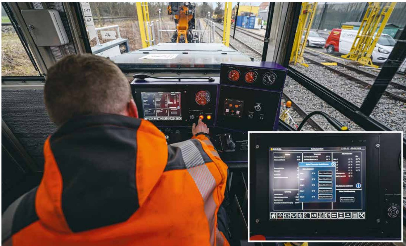
Fig. 4: The aluminium cab offers space for two identical driver's workstations plus five people. Large glass panes provide a generous view of areas around the vehicle.
