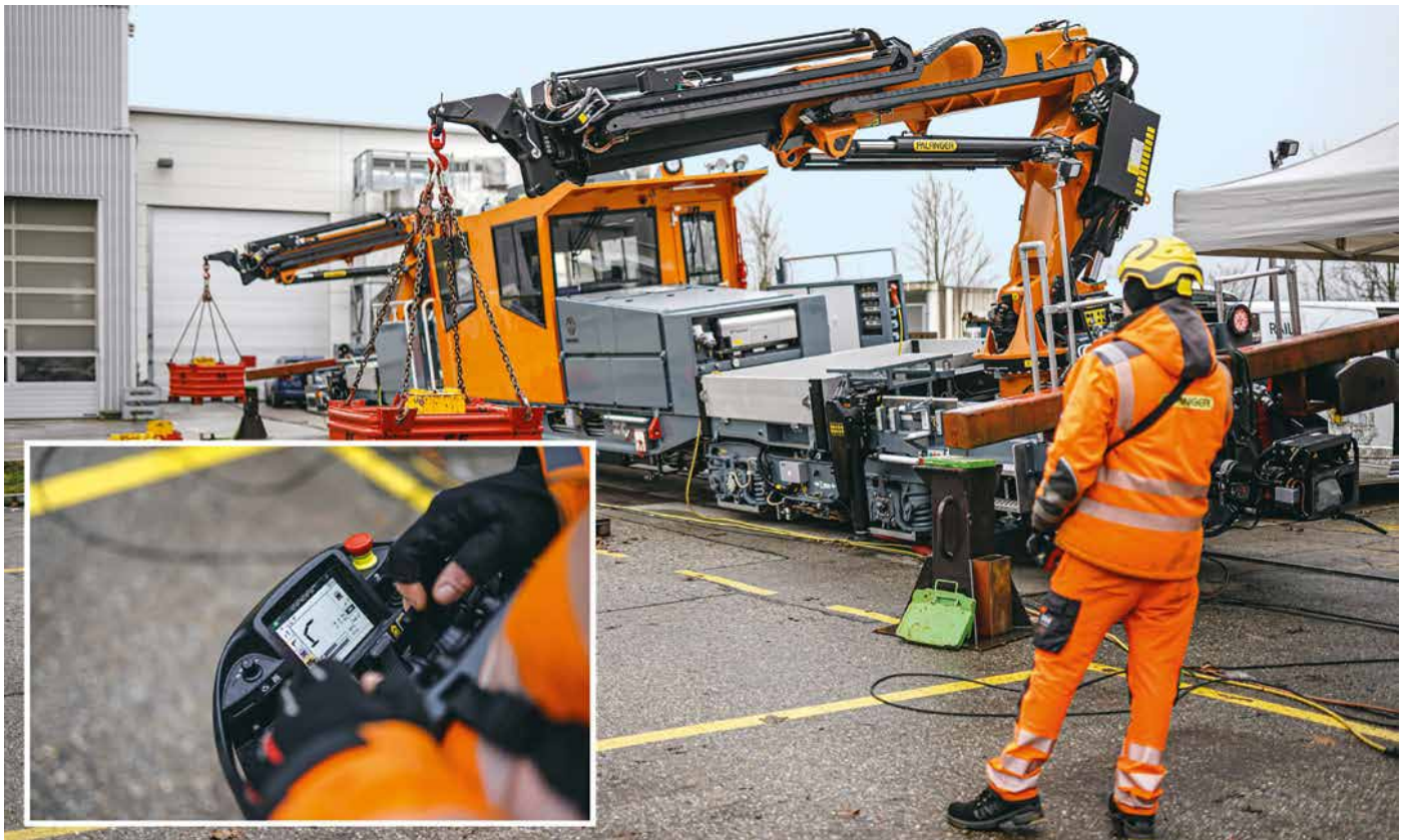
Fig. 3: Stability test in superelevation with simultaneous, remote-controlled crane operation.
