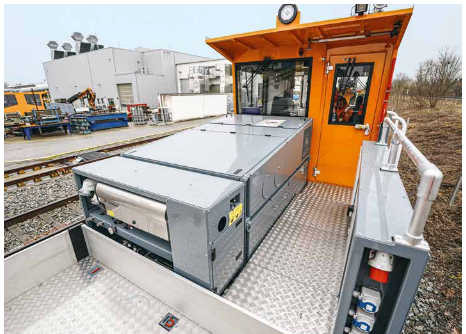
Fig. 2: The battery pack is dimensioned for exactly 3.5 hours of battery-powered working.
