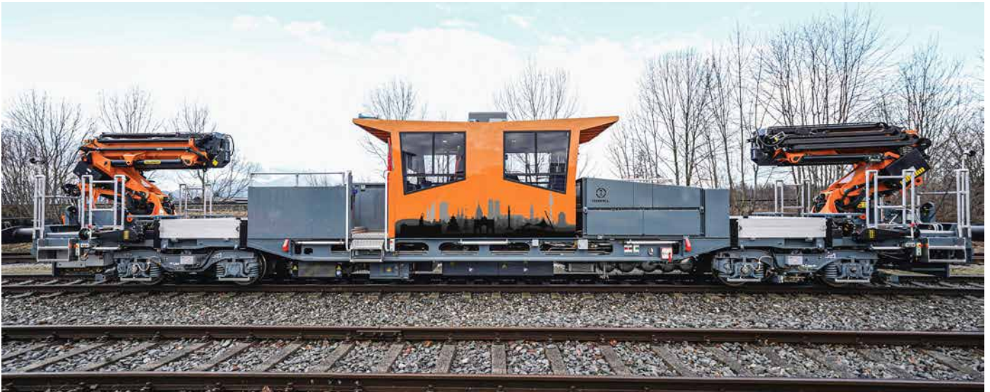
Fig. 1: With its symmetric design, the electric track maintenance vehicle for Munich's public transport company is designed for bidirectional operation.
