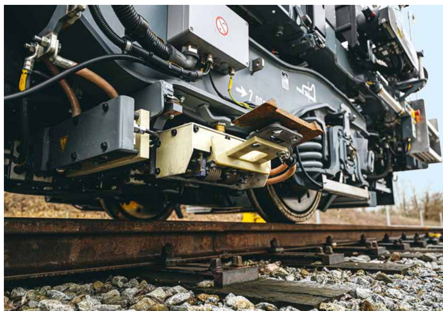
Fig. 5: The pantograph for the side conductor rail is attached diagonally to the bogie and can be retracted without infringing the structure gauge.
