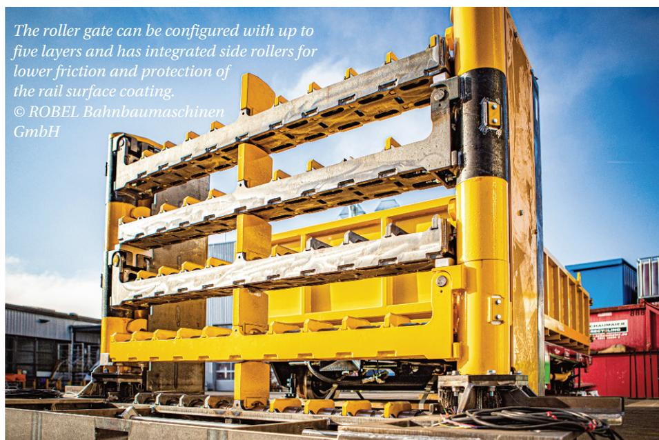
*The roller gate can be configured with up to five layers and has integrated side rollers for lower friction and protection of the rail surface coating.*
