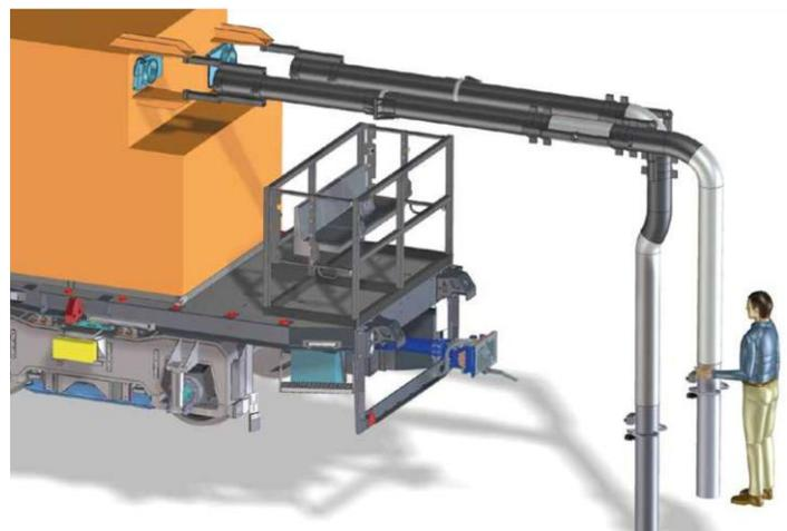
**Operators can unroll separate suction hoses to up to 20 metres and so can reach areas that are otherwise difficult to access, such as recesses and shelters next to the track.**
