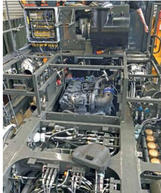
The track vehicles for Norway were fitted with new engines and fully rewired.
