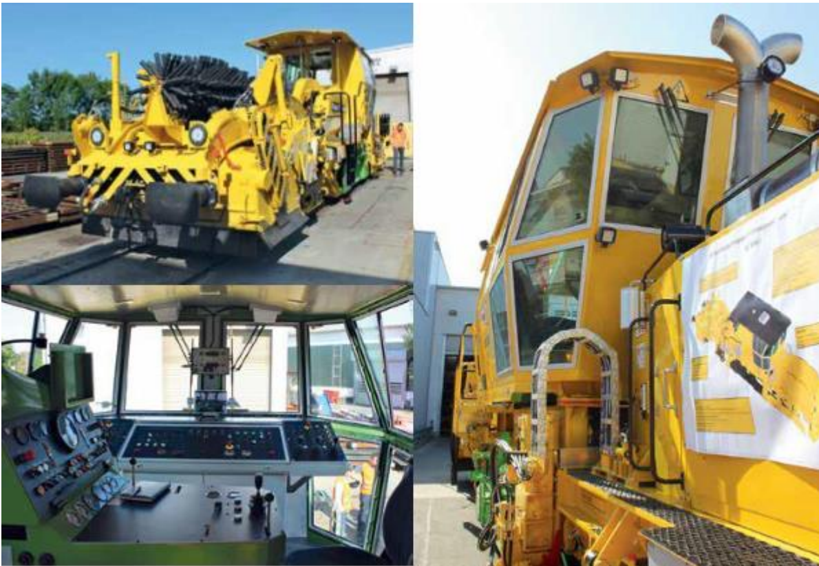
In the course of 2019, a quick-action ballast distributing and profiling machine (SSP) from the track construction company H. F. Wiebe was retrofitted at Robel Bahnbaumaschinen GmbH for many more years of service life. The machine was not only fully reconditioned (above left) but was also fitted with a new cab with a new driver's and operator's desk (bottom left) as well as numerous new windows for an even better all-round view of the work site (right).
