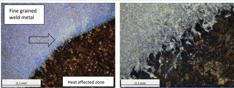
**Fig. 5:** Metallurgical examinations of etched sample rail sections with 3% HNO<sub>3</sub> show clearly a finer grained ground face at the transition from the weld metal to the heat affected zone.
