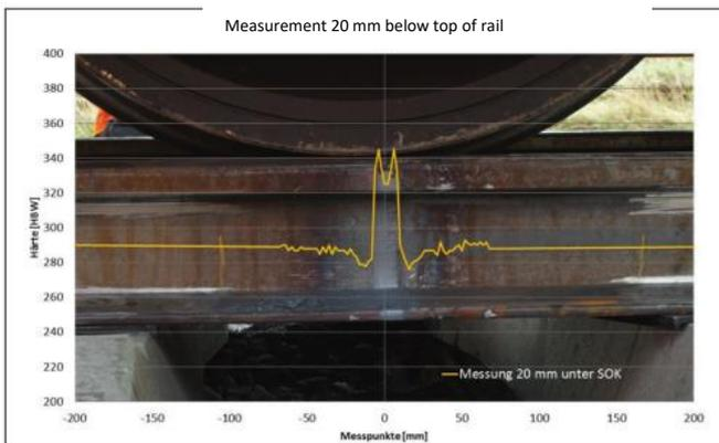
**Fig.3:** Maximum strength: The filler materials used for automated welding harden the material and thus reduce the heat affected zone – this is not impaired by the wheel.
