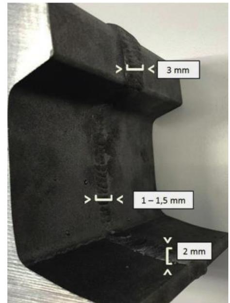
**Fig. 7:** The projecting weld bead of an automated joint welding at the current state of development: Sufficient material for finish grinding is available at the railhead; no further work is required at the rest of the rail.
