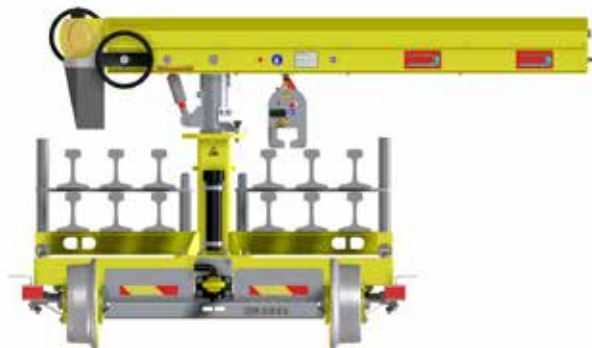
Loading diagram with 12 rails max. on 2 levels
